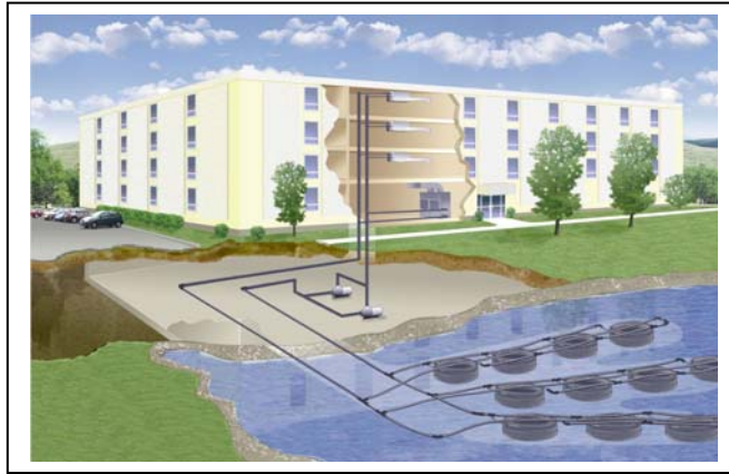
Figure 24 – Surface Water Loop
